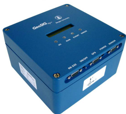
Figure 1. Ambient noise recording systems, used in our experiment: a) GBV-316 data acquisition system; b) X-Tremer 45 smartphone accelerometer
