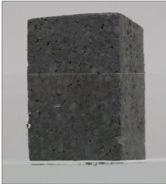
Figure 21. A lightweight body made of expanded polystyrene floating as if on a solid surface
