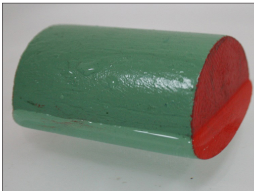
Figure 10.3. The stable floating position of the tallest cylinder
