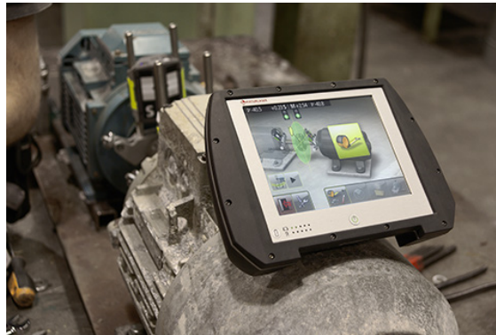
Figure 2. Laser shaft laser alignment (ACOEM Fixturelaser 2020)
